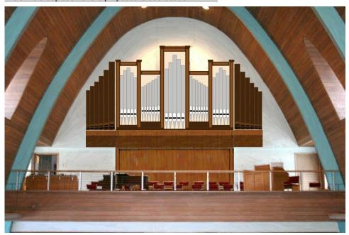
Rene Marceau and Robert Collins are working together to build all new wind chests and casework for the project. The pipe organ will employ MIDI controlled direct-electric stop action and run on 5" of wind. Tonal finishing will be completed by Rene Marceau.
